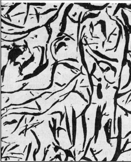
Photomicrograph of gray cast iron (100x) showing carbon in the form of graphite flakes.
